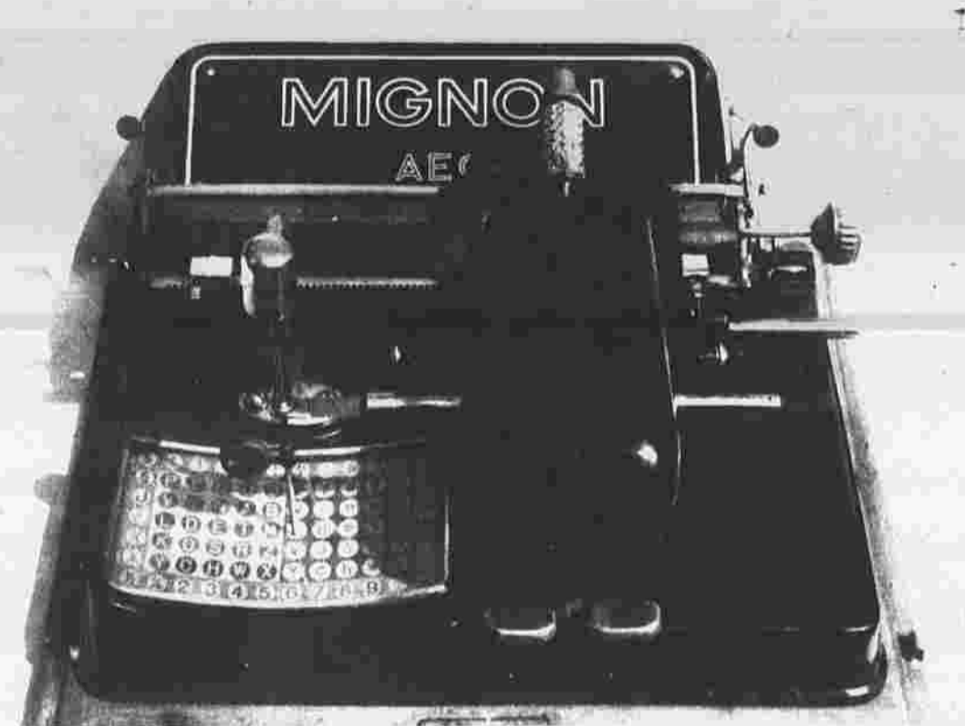
MIGNON IS AN INDEX TYPEWRITER sold from 1903 to 1940 in Europe
